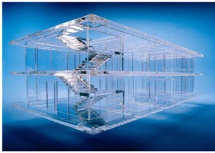
Figure 1. Model of multi-compartment structure used in the water-tank experiments.
